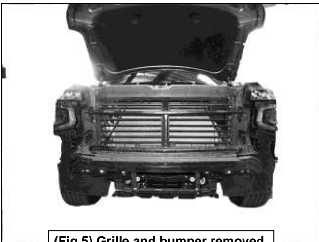
(Fig 5) Grille and bumper removed
